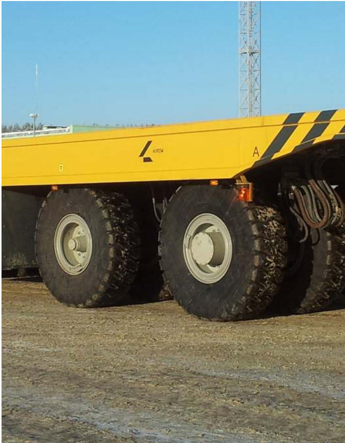
↑ Large tyres ensure good maneuverability on uneven roads, a permanent ground contact of all tyres and increases the driving comfort
