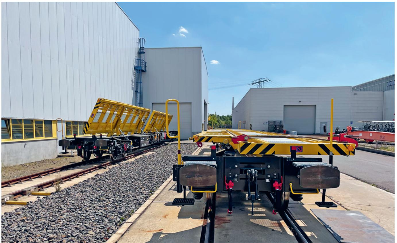
The load fixation in particular can be variably adapted to local safety regulations.
