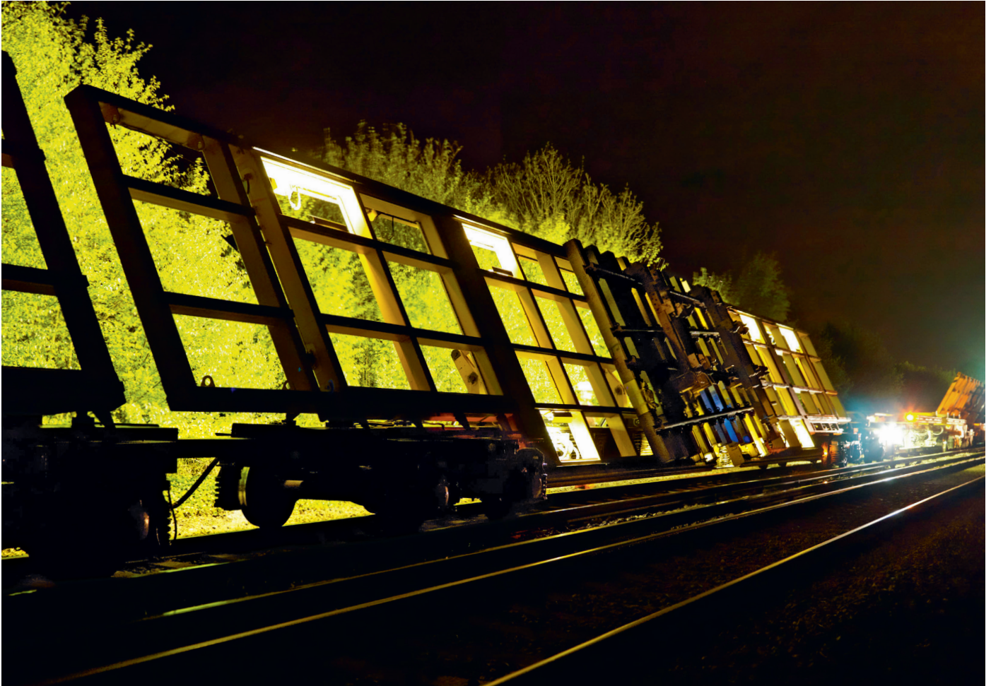
↑ Cross and Connecting Beams fix the loaded switch section on the Switch Tilter
