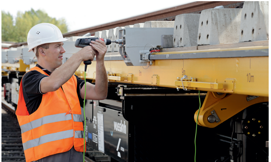
Manual Operation of the load fixing system from the ground
