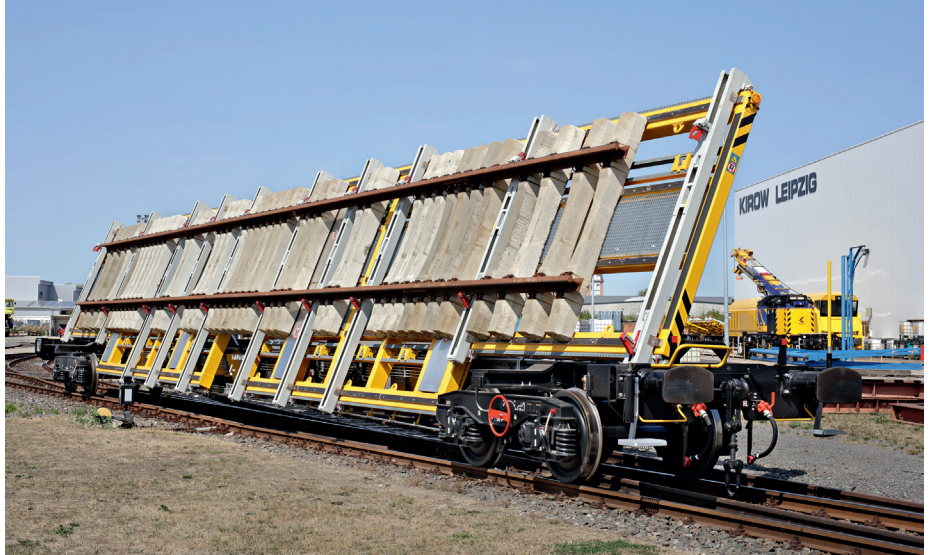
Kirow Switch Tilter with manual-mechanical load fixing system for Vossloh Logistics
