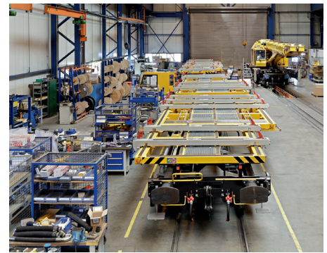
↑ Switch Tilter in the assembly hall
