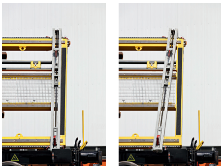
Manually movable and turnable Connecting Beams
