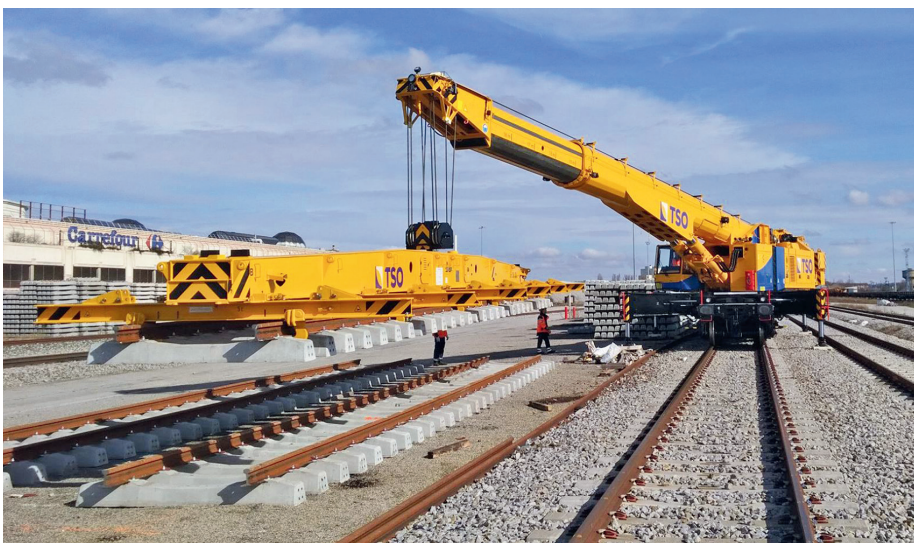
Switch segments can be directly fixed to the Switch Handler using the integrated load hooks
