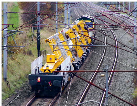
Minimised loading height guarantees transport under overhead lines
