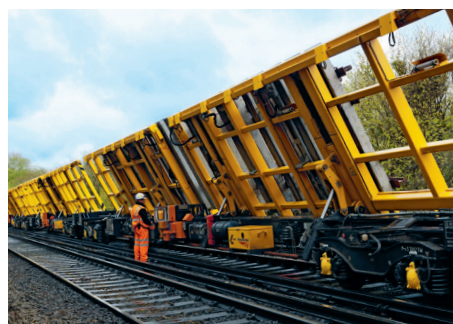
↑ Just one operator starts the Switch Tilters
