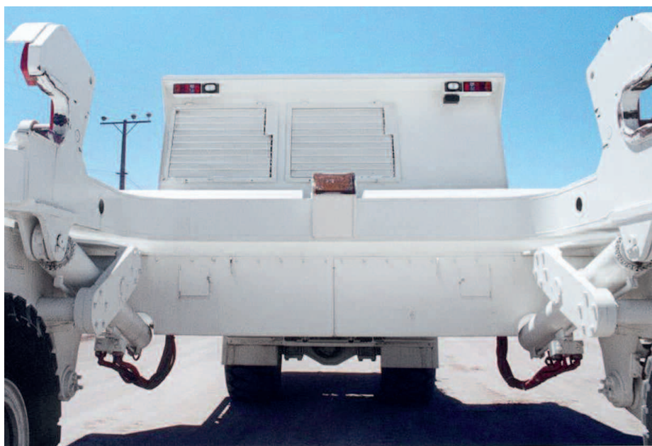
↑ Extensive protective covers on Slag Taurus U
