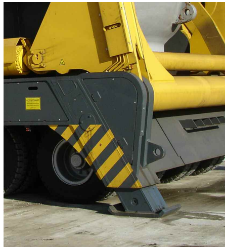
↑ Integrated support with protected support cylinder
