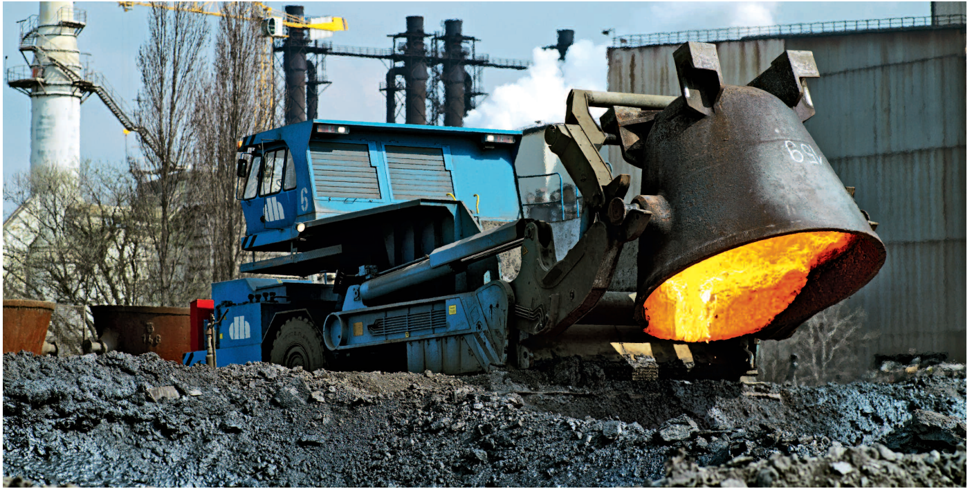
↑ Slag Taurus P with conventional tipping system
