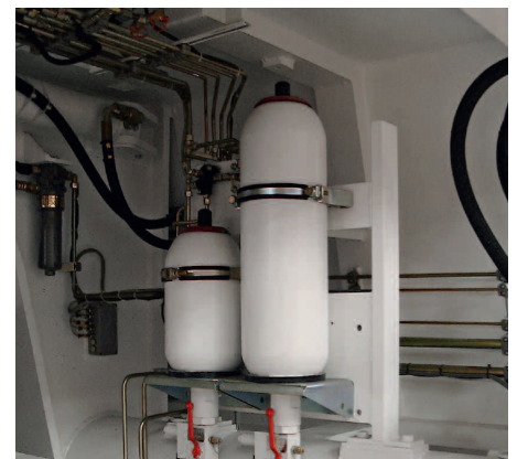
↑ Hydro-pneumatic accumulator for brake system
