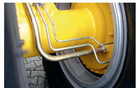
↑ Wet multi-disc brake in enclosed design
