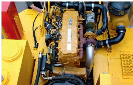
↑ Large-sized engine hood: optimal access for maintenance
