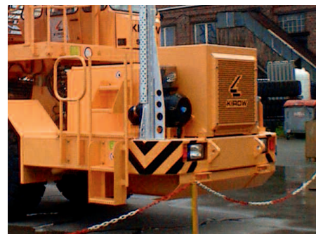
↑ Option vertical exhaust pipe: for indoor operation
