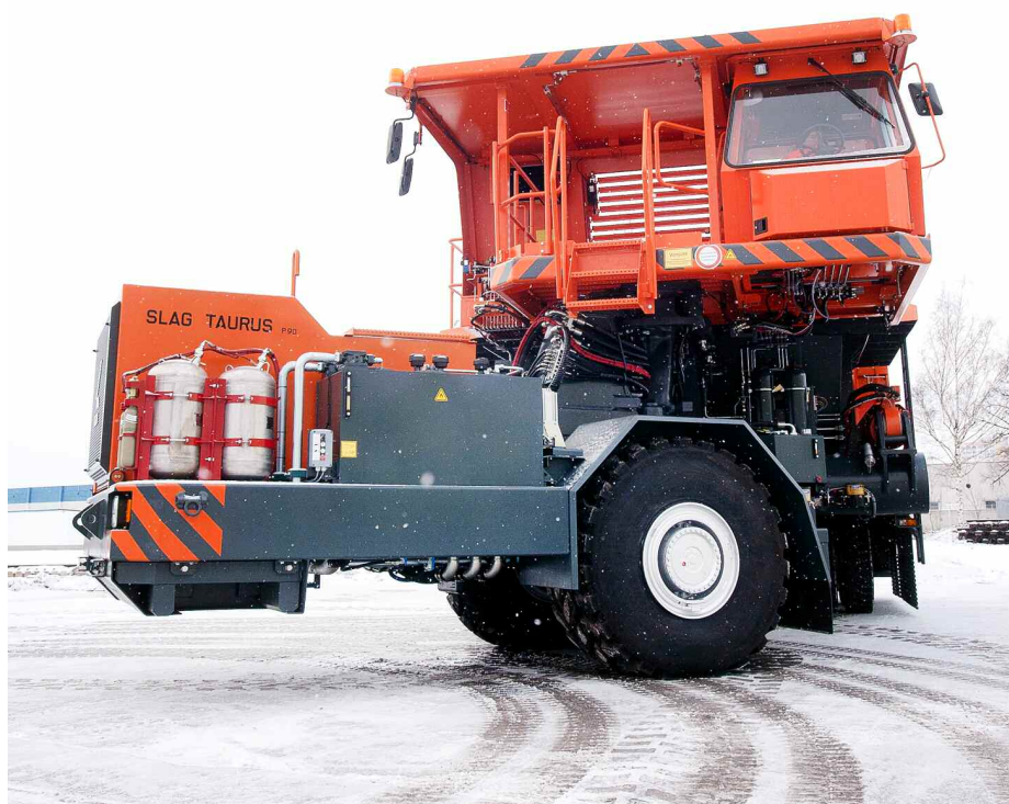
↑ Optimal arrangement of driver's cabin: independent of steering movements
