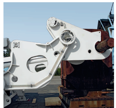
↑ Slag Taurus P with lever linkage dumping system
