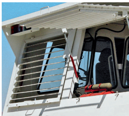
↑ Large-sized observation window at cab protection canopy
