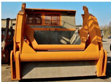
↑ Extensive protective covers on Slag Taurus P
