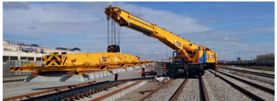
↑ Switch panels can be directly fixed to the Switch Handler by using the integrated load hooks
