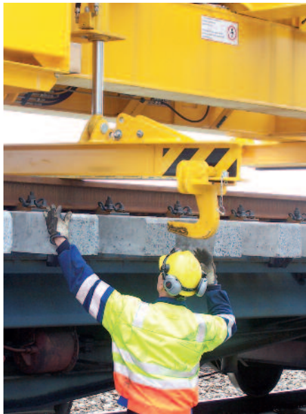
↑ Lifting hooks can be operated from the ground
