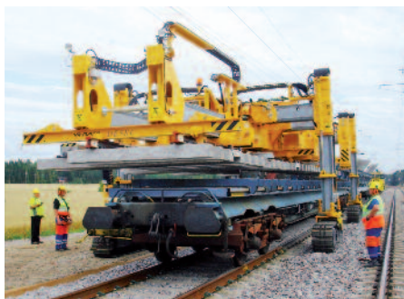
↑ Switch transport wagon tilted down for unloading by Tracklayer
