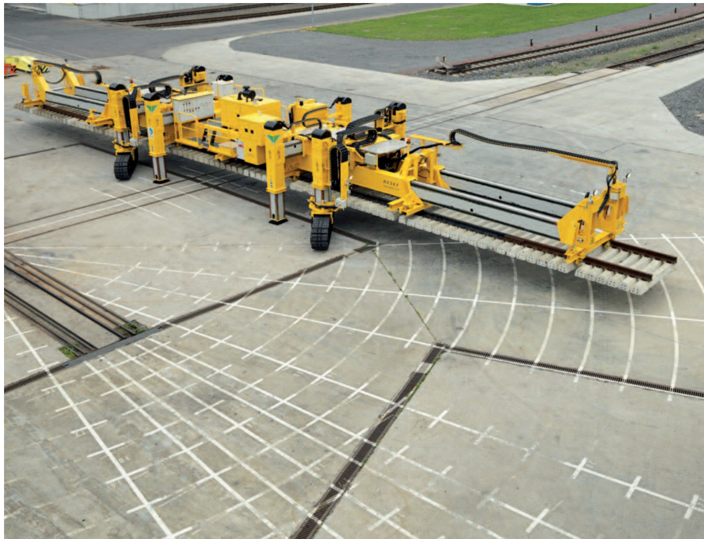
↑ Sidestepping, steering and change of direction without lowering the load
