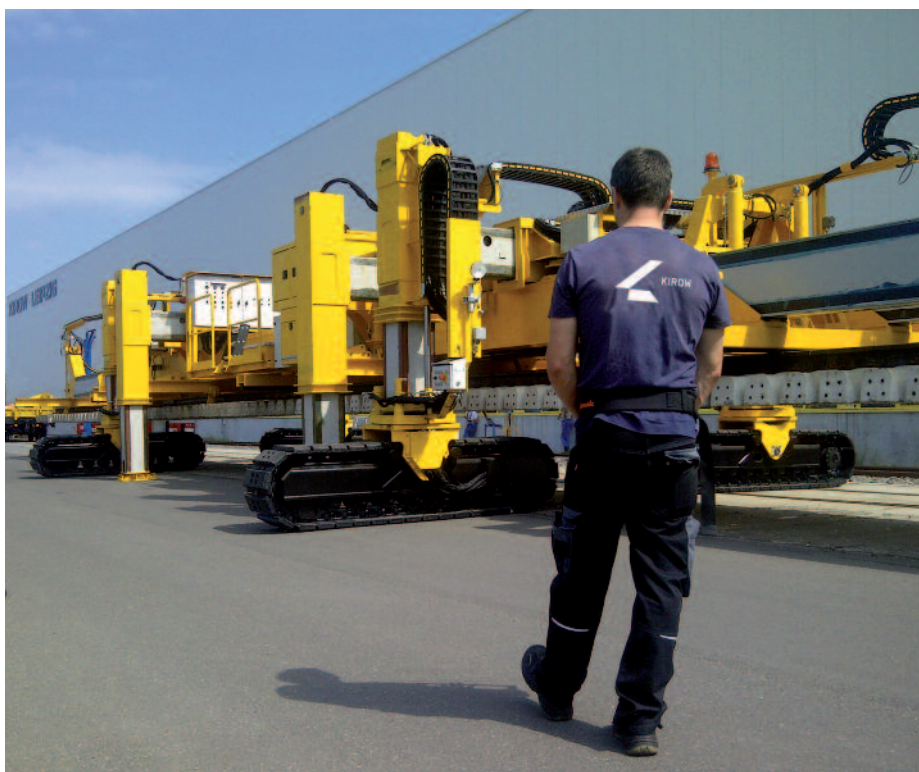
Just one operator controls the DESEC Tracklayer by radio remote control
