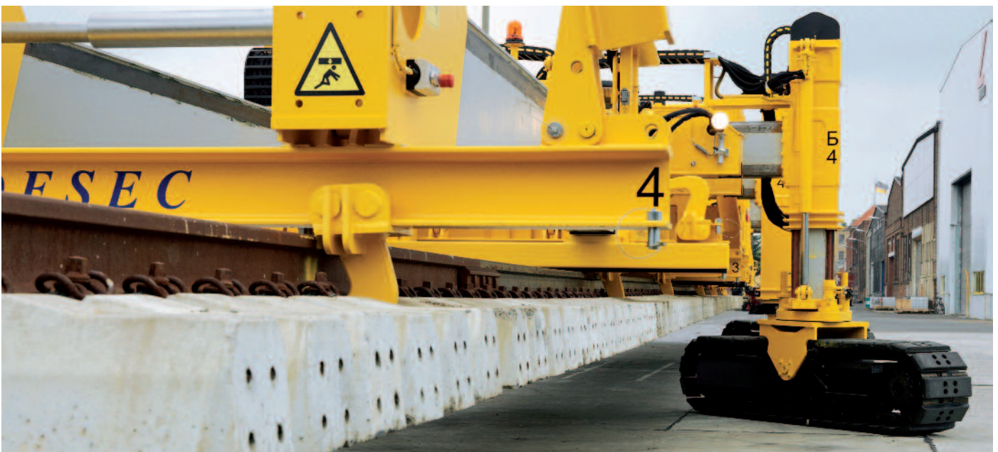
↑ Switch panel is carried without bending or twisting
