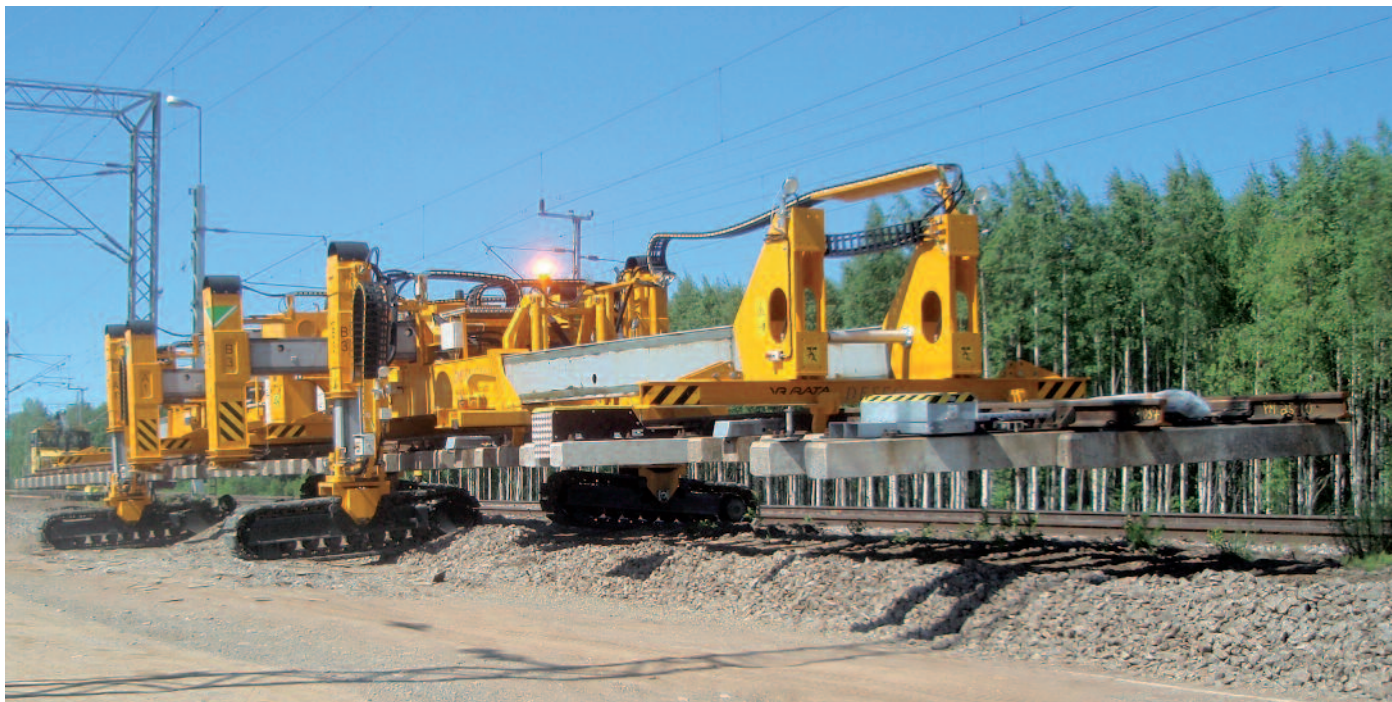
↑ Panel pick up from the trackside
