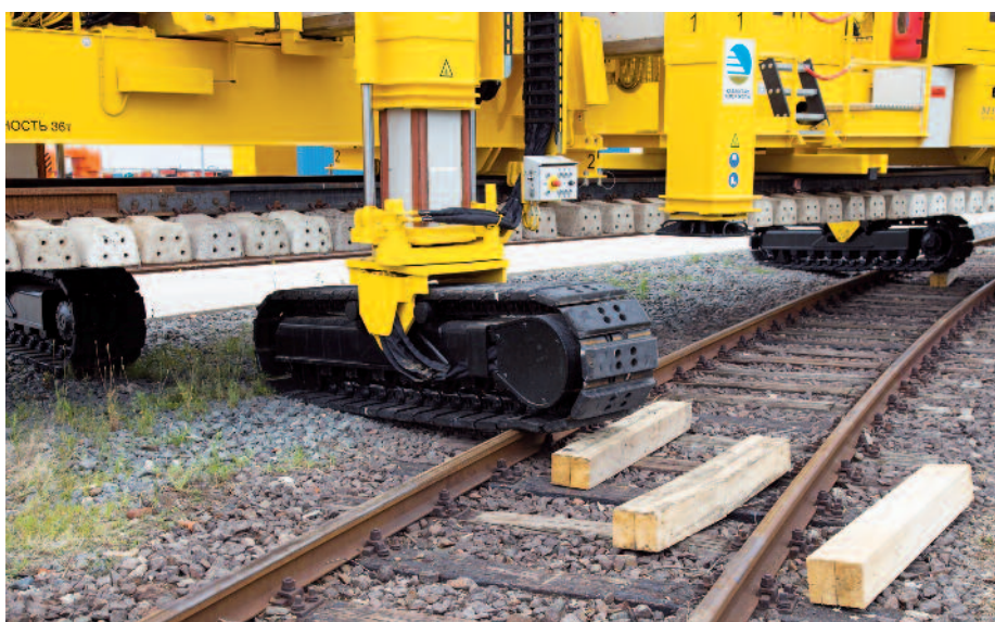
↑ Rubber coated crawler pads for driving in the railway environment
