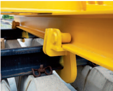
↑ Load is grabbed by lifting hooks underneath the rail foot
