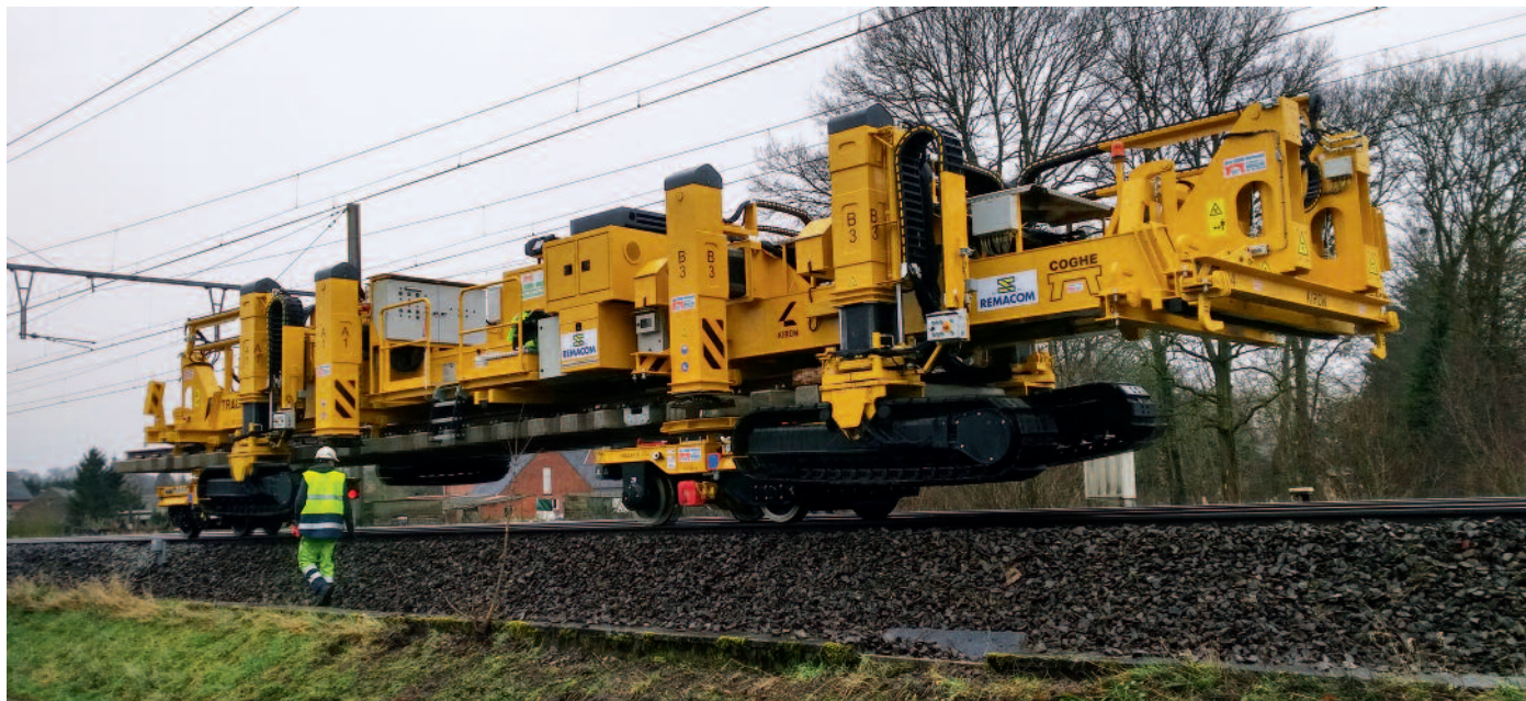
Tracklayer with loaded turnout panel on trolleys during travel to the installation site
