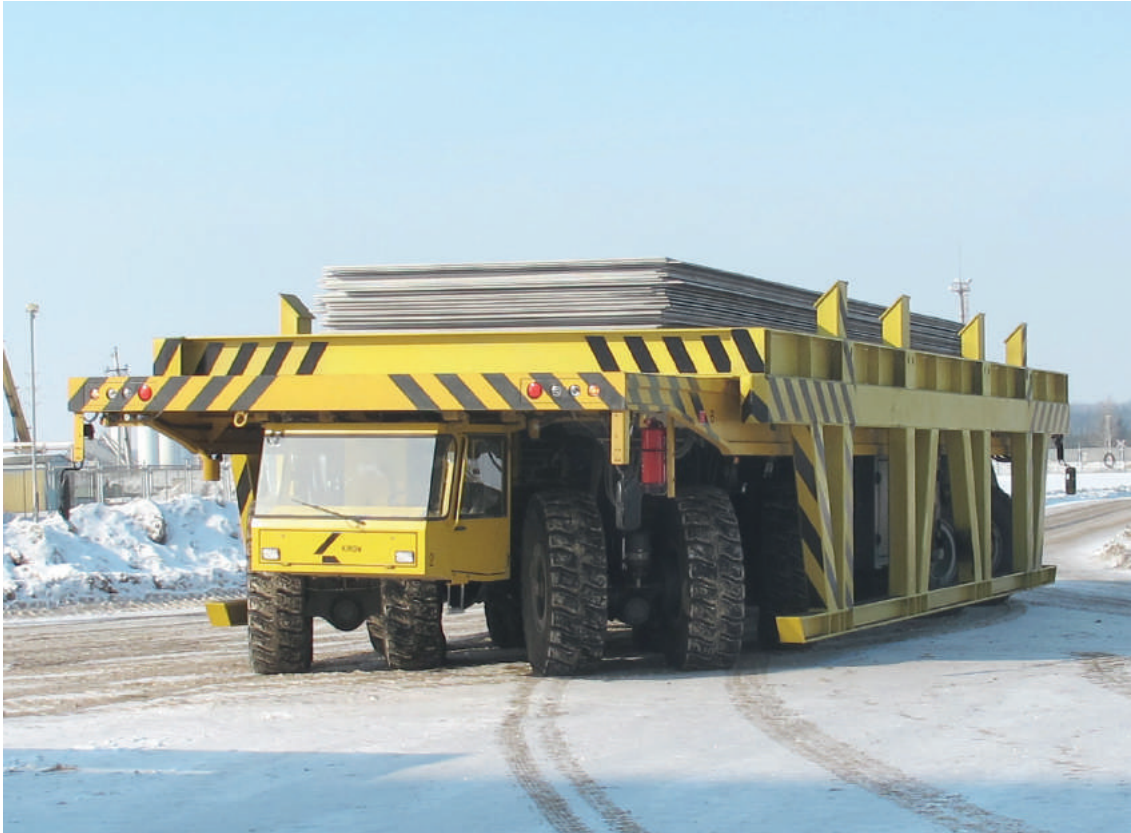
↑ Multi Mover M transporting flat material
