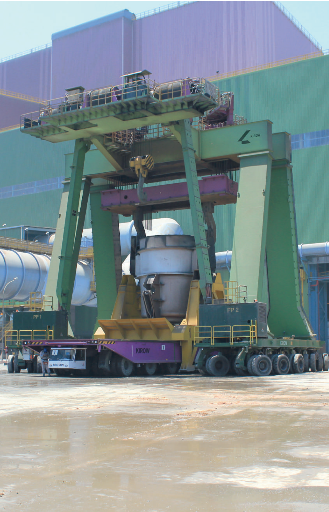
↗ A Multi Mover Y transferring a pig-iron ladle to the Multi Mover M
