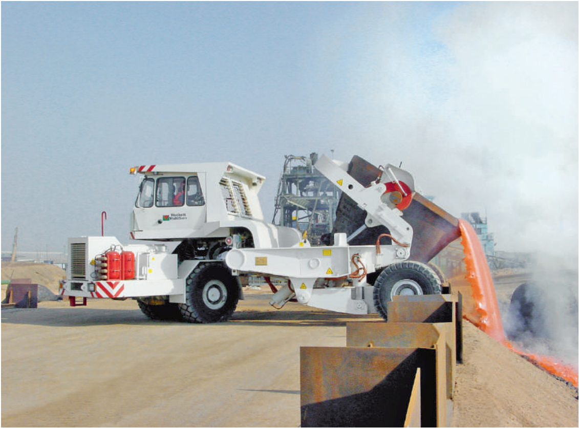
↑ The Slag Taurus U with U-frame steel structure
